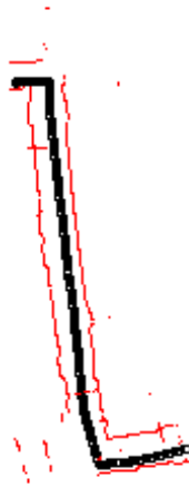
Figure 6.6 An experiment result of a learned path. The black circles are spots specified by the coordinates obtained from the odometer and the red lines are the distances obtained from ultrasonic sensors.
