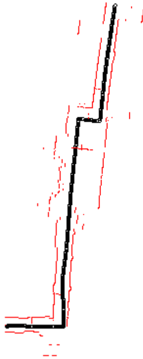
Figure 6.12 An experiment result of a navigation path. The black circles are spots specified by coordinates obtained from the odometer and the red lines are the walls plotted according to the distances obtained from the ultrasonic sensors.
