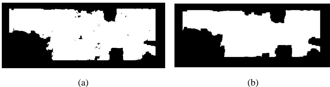
Figure 4.3 An example of refining a map. (a) A rough map. (b) A complete map after applying the erosion and dilation operations.
