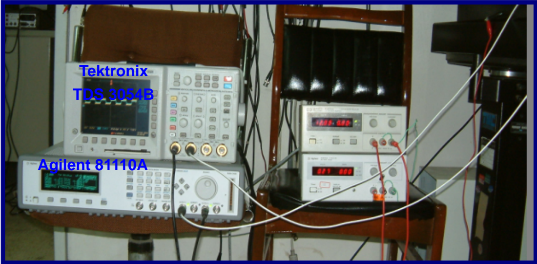
Fig. 3.13 Instruments for measuring class-B output buffer.
