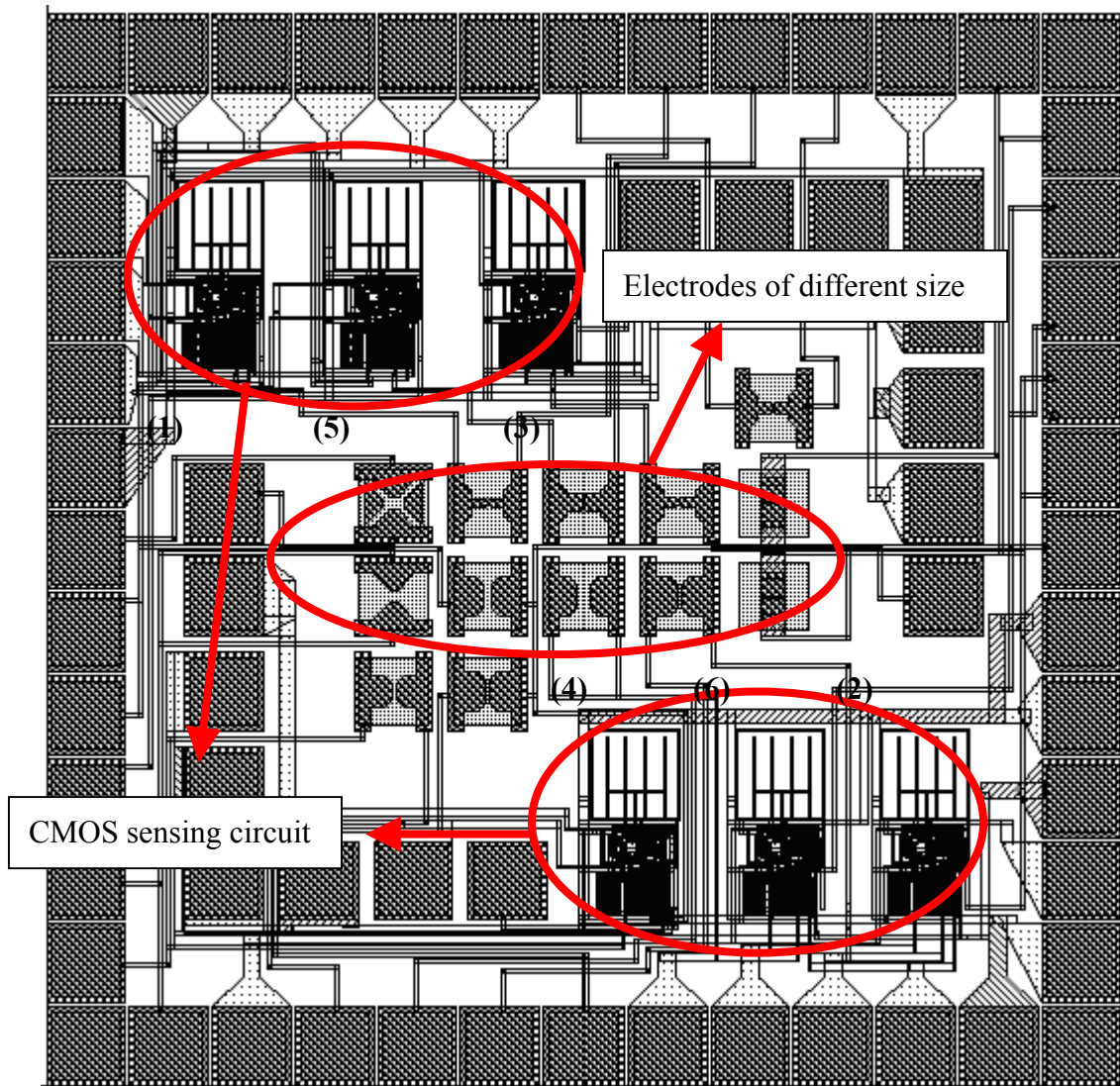
Fig. 4.1. The layout of the CMOS sensing chip is shown above. The chip is 1.35 mm * 1.35 mm and has 48 pins. There are six identical CMOS sensing circuits, (1)~(6)
