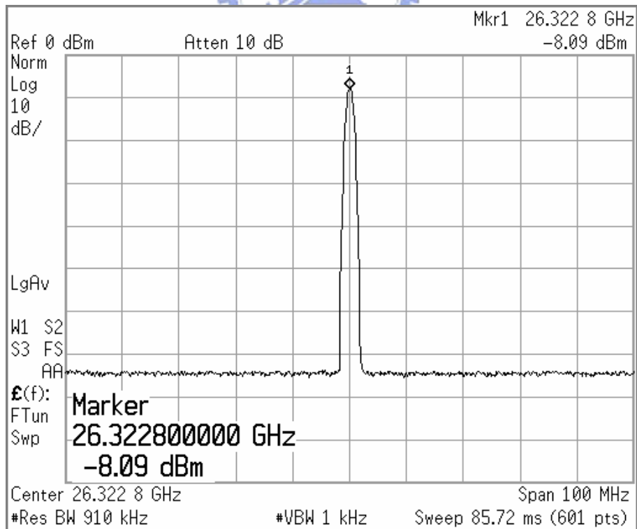
Fig. 2.23 Measured output spectrum of the fabricated K-band ILFT under locked condition with probe and cable losses, V_{BIAS} of 0.56 V, and input power of 4 dBm.
