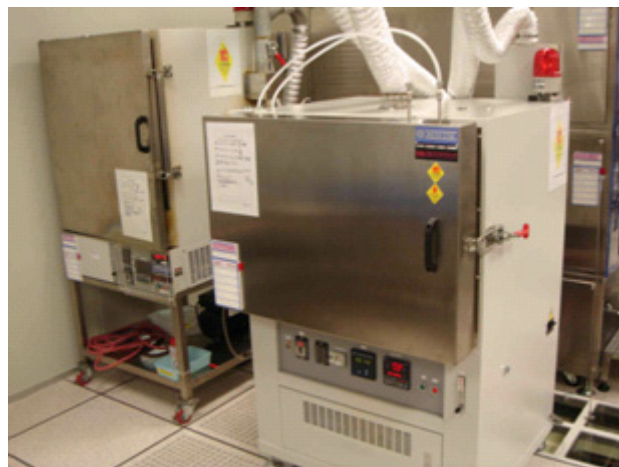
Fig2.19 BCB / PI dielectric layer Oven
