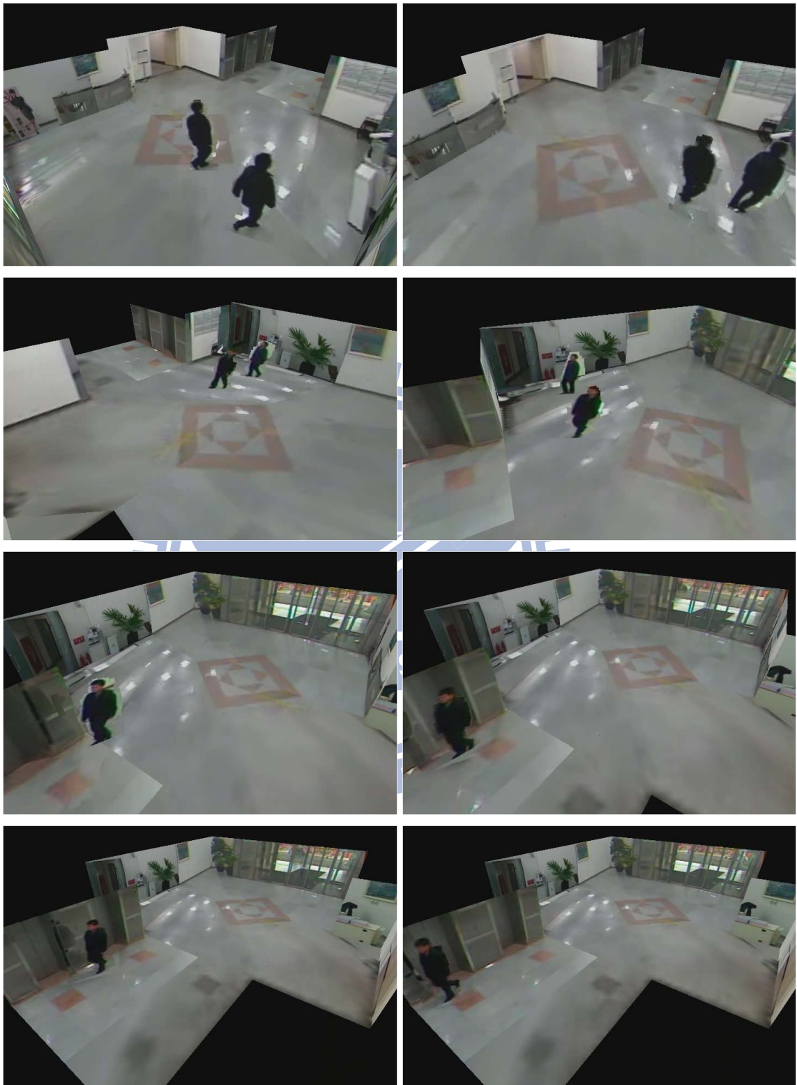
Figure 4.15: Auto-tracking of targets. The viewpoint of the operator auto-switch according the number of people in the monitored area. Two people in the view walk across the lobby and the viewpoint keeps track of targets.
