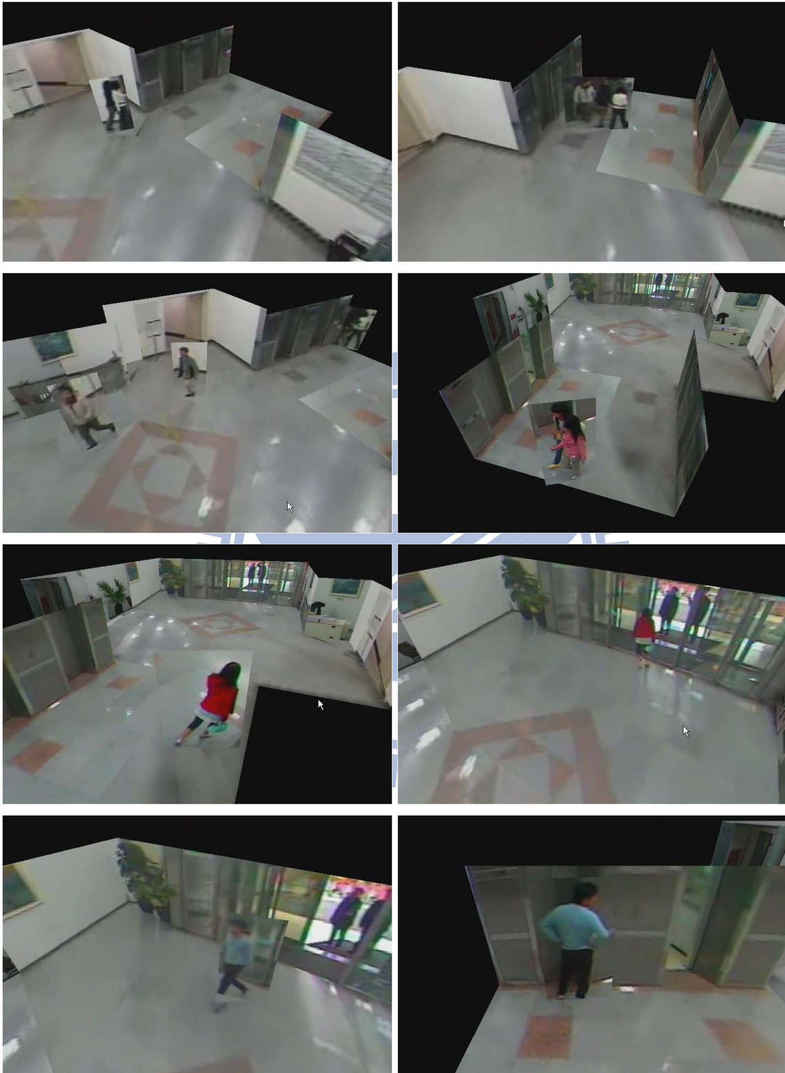
Figure 4.12: Results of the immersive monitoring. We can observe pedestrians with any viewpoint in the monitored area. The billboards are always facing to the viewpoint.
