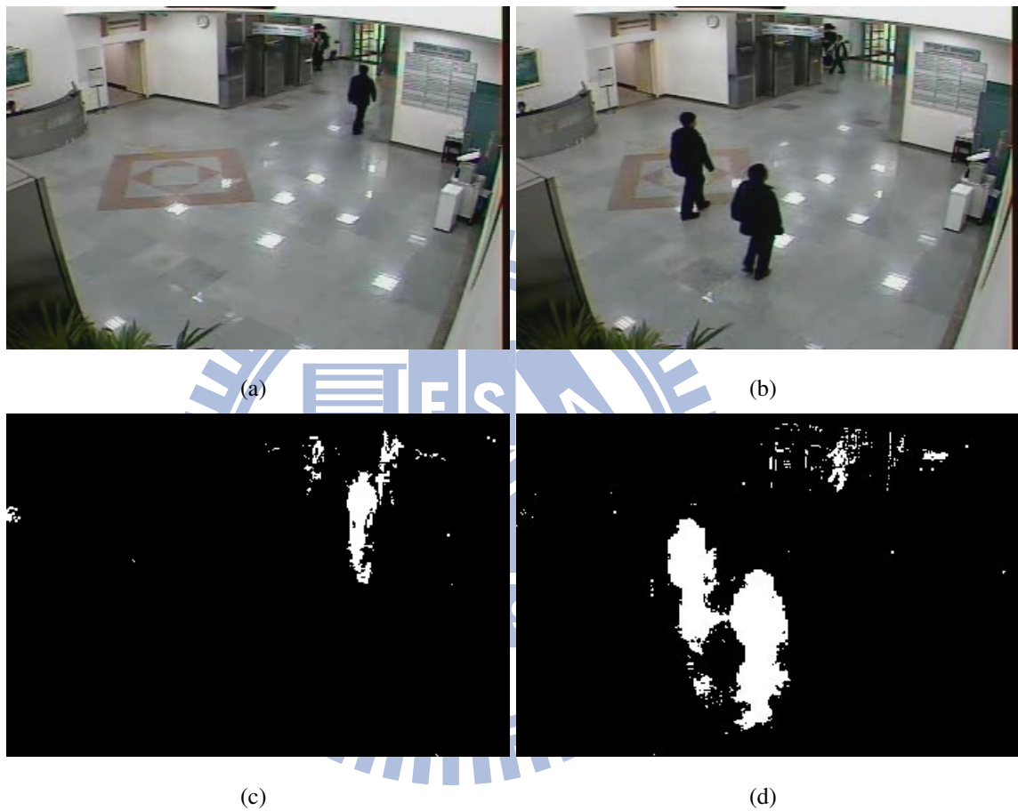
Figure 3.4: The detection of foreground objects by codebook algorithm. (a) A frame from the camera. (a) Another frame from the camera. (a) A foreground mask. (a) Another foreground mask.
