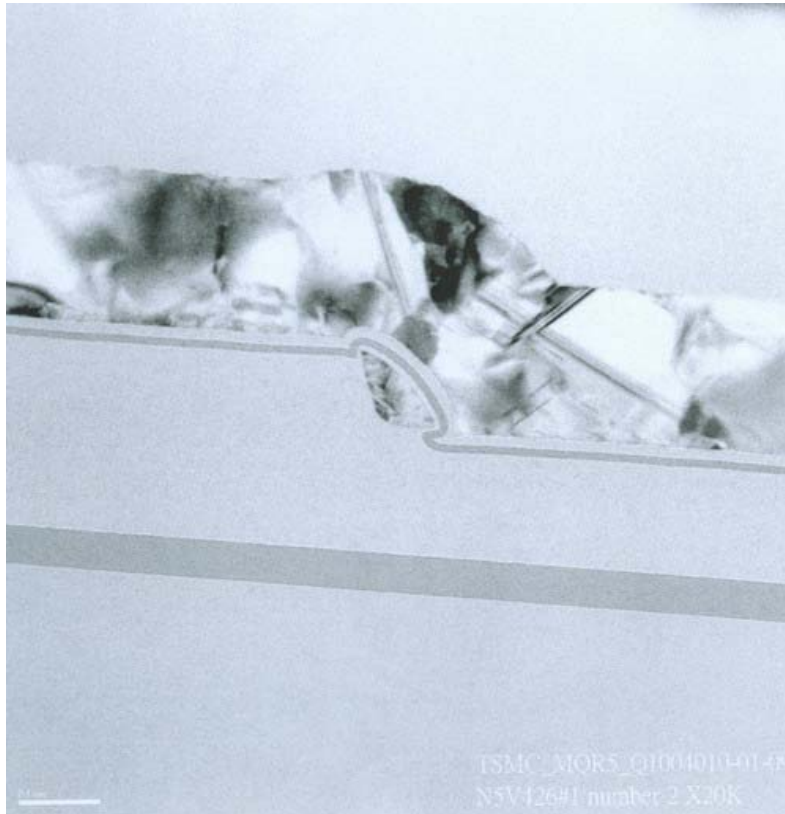
Fig. 2-11 The cross-section TEM image after patterning gate for the omega gate structure.
