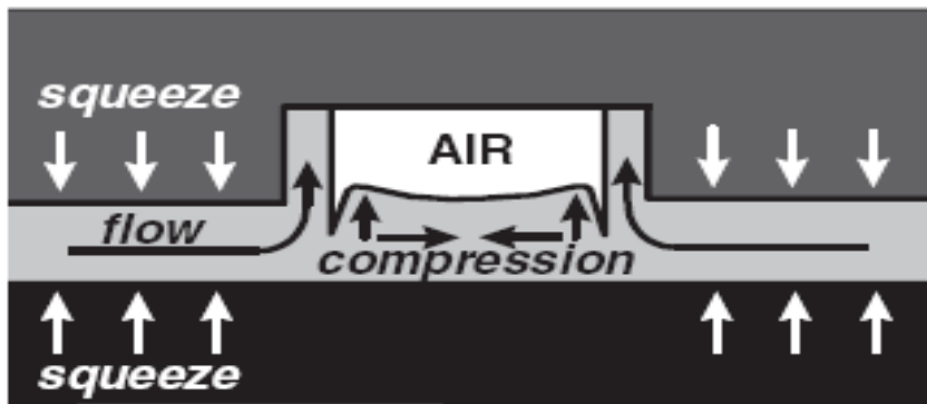
Figure 3.16: A schematic representation of squeeze flow of a polymer into a stamp cavity [3-9].
