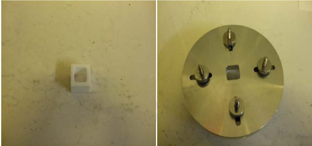
Figure 2. 5Teflon container (left) and stainless steel mold (right) used to fabricate the soft stamp.
