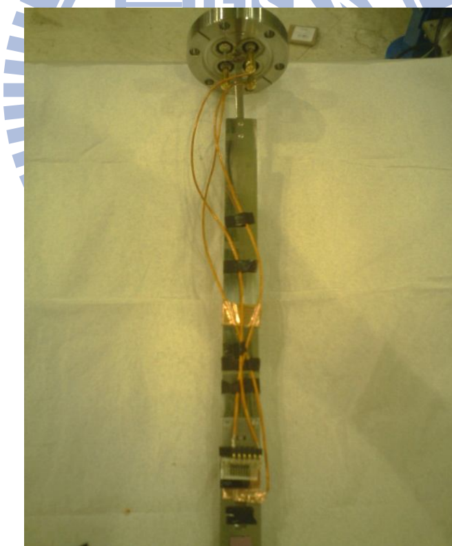
Fig. 2-8 Outlook of sample rod which is connect to the in-situ measure sample.
