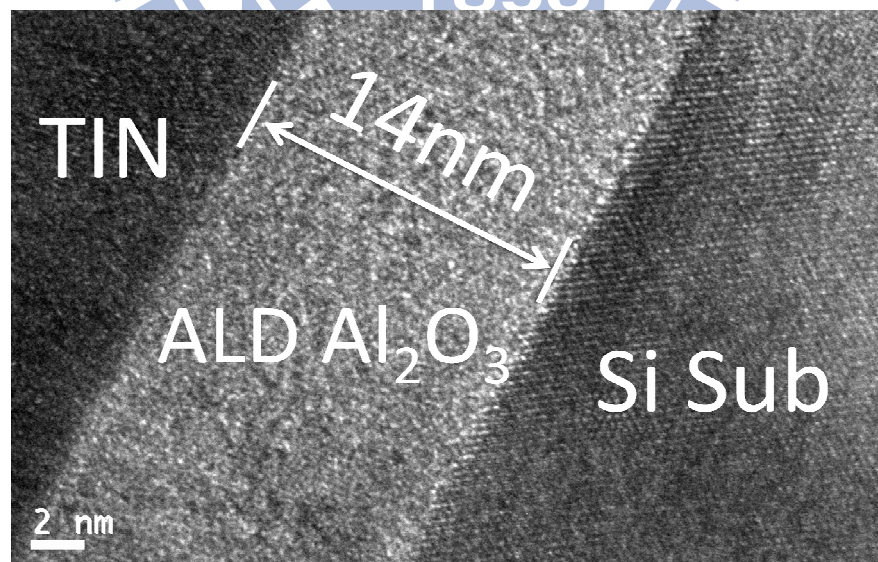
Fig. 3-6: Cross section of MOCVD \text{Al}_2\text{O}_3 with IL and rough surface between the TiN.
