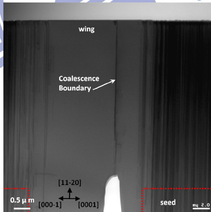
Figure 5.06. The TEM images of a -plane GaN grown by MOCVD using TELOG technique under the V/III ratio of 72 and 980°C. The corresponding coalescence boundary between + c -plane and - c -plane is depicted.
