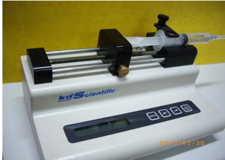
Fig. 3-8. Controllable syringe pump.
