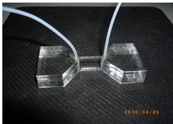
Fig. 3-3. The plastic used to press the PDMS microfluidic. An inlet and an outlet tubes are connected to the microfluidic for flowing the test solution during testing.
