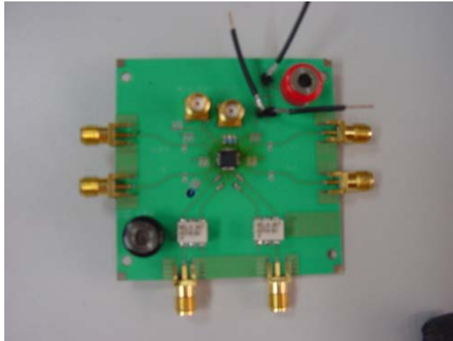
Fig. 99 Overview of Chip On PCB (TXFE-LP)
