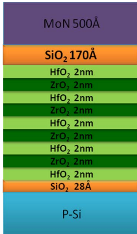
Fig.4-1 Cross section view of MoN/SiO 2 /HfO 2 -ZrO 2 /SiO 2 /Si structure which was not patterned.
