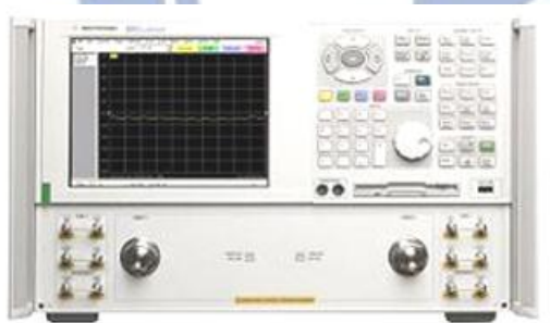
Fig. 3.7 4 port S-parameters measurement setup including Agilent PNA E8364B, test set N4421, bias-Tee, RF cables, and adapters with 2.4mm spec. for high frequency measurement up to 50 GHz.
