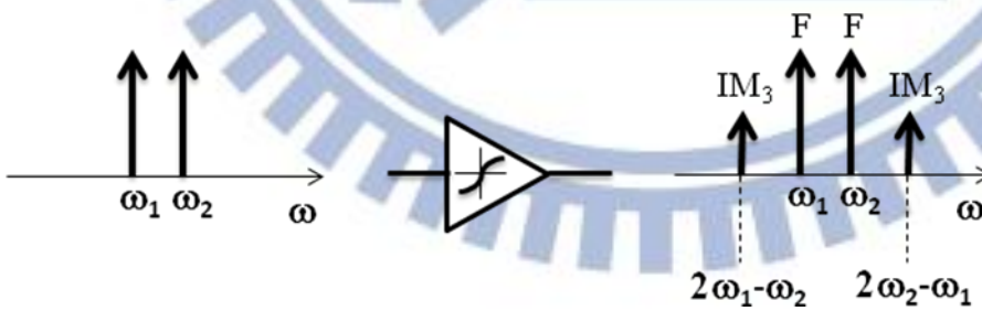
Fig. 2.6 Intermodulation in a nonlinear system
