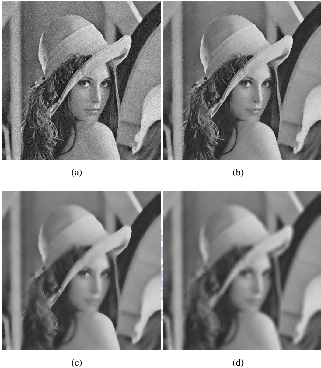
Fig. 2.4. Smoothing results of BF with different range parameter \sigma_r (a) noisy image, (b) \sigma_r=25 , (c) \sigma_r=100 , (d) \sigma_r= very large (GF).
