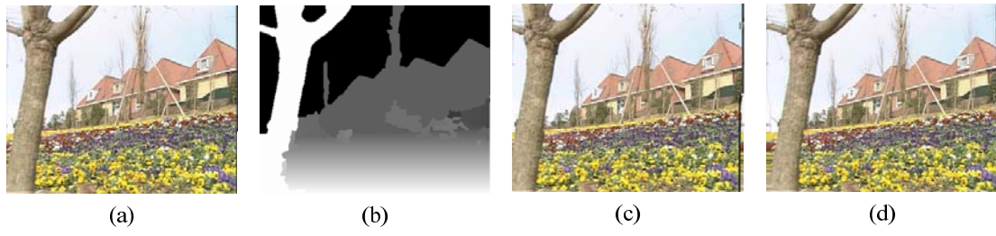
Fig. 3.21. The result of DIBR algorithm. (a) Original image. (b) Disparity map. (c) Rendered left view. (d) Rendered right view.
