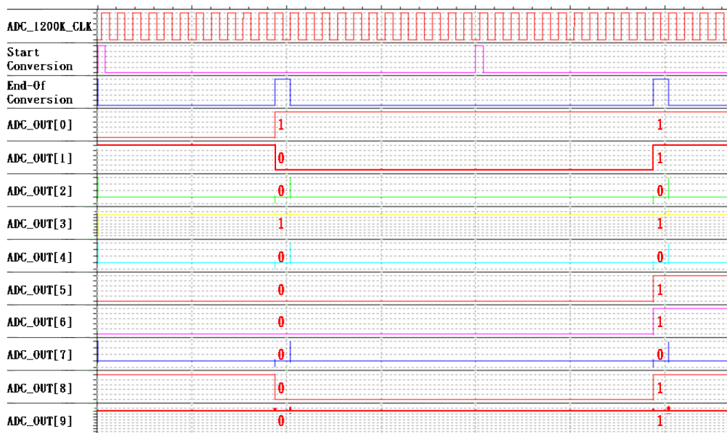
Figure 3.2 Analog-to-digital conversion (ADC) simulation waveform
