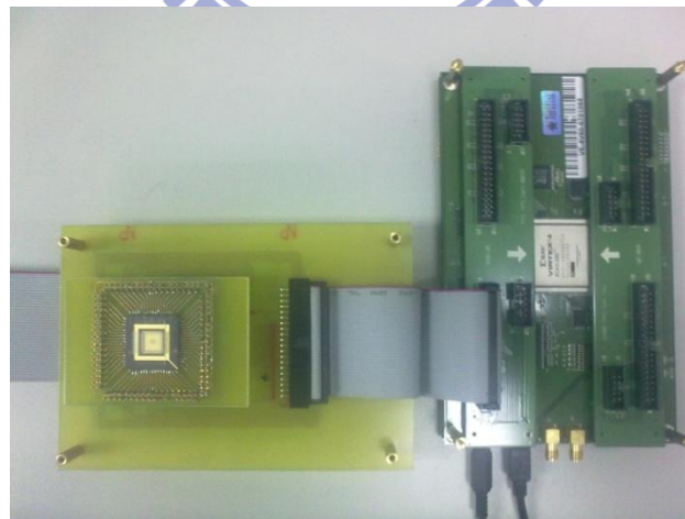
Figure 2.40 Connection between the FPGA board and the PCB
