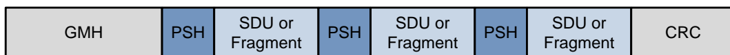
Figure 2-3: Examples of the Ordering of Payload and Sub-headers in a MAC PDU
