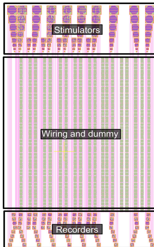
Figure 2.3 Layout view of the microelectrode chip.
