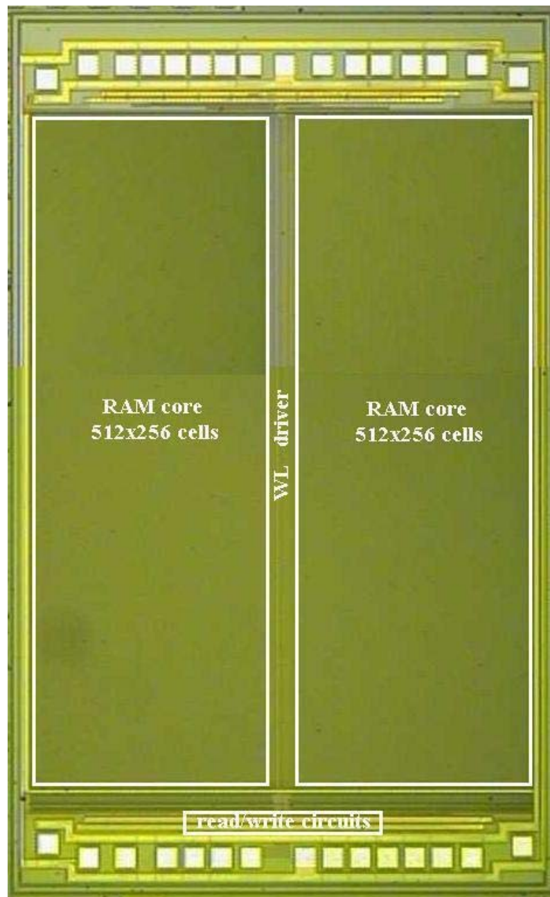
Fig.49 A photomicrograph of 32Kx8 SRAM
