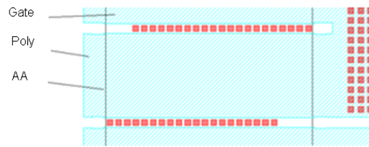
Figure 3.15: Correct mask algorithm for implant layer and the corresponding virtual mask set GDS with no extra generated implant layer.
