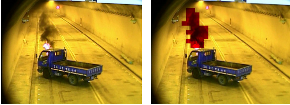
(a) Smoke objects in a tunnel
