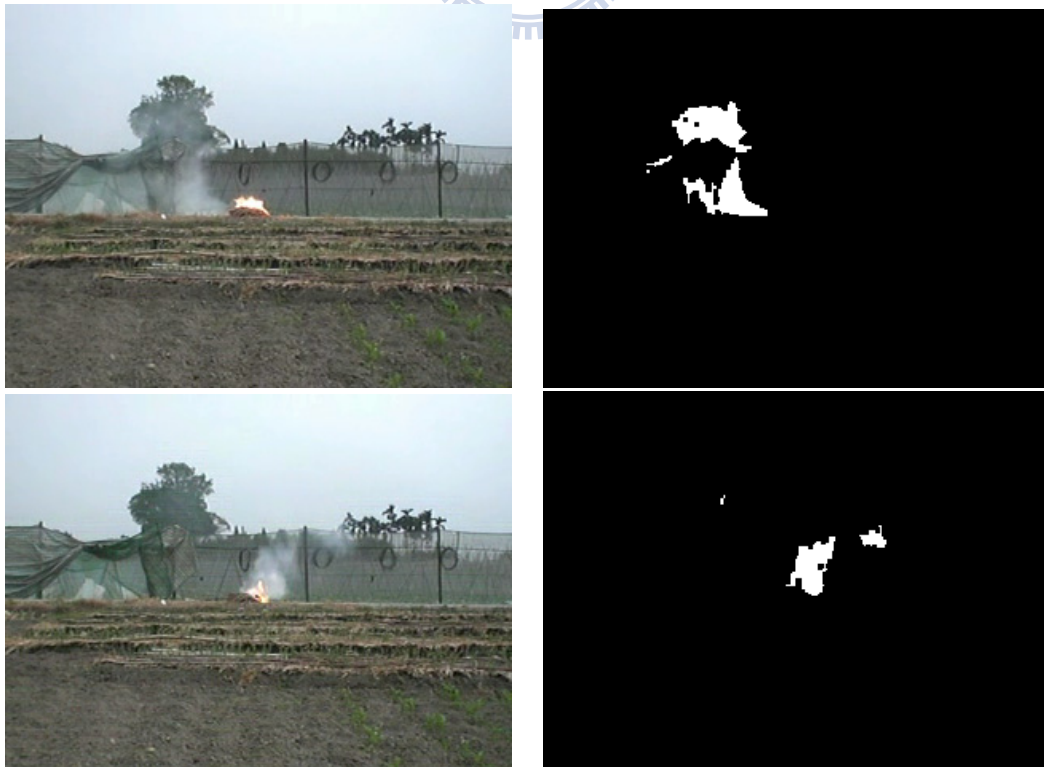
Fig. 3-5 Smoke regions come into existence and disappear continuously
