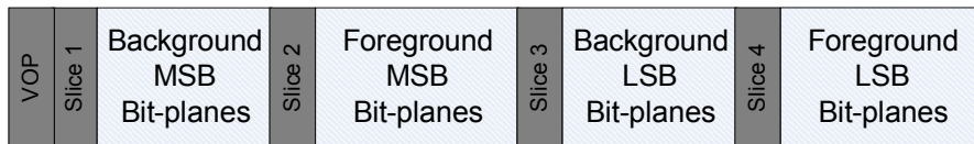
Figure 4.18: Flexible slice structure with fine granularity.
