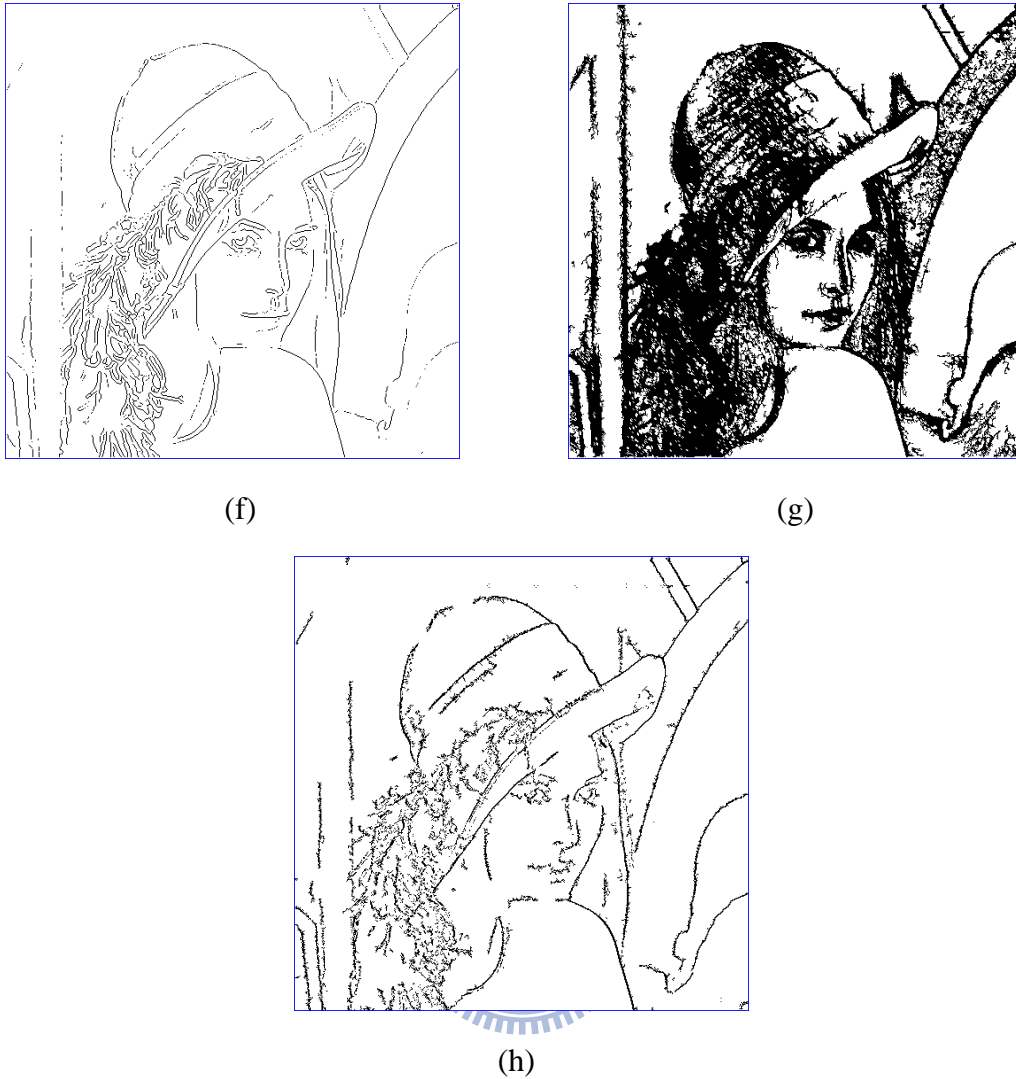
Fig. 4.17. Edge detection results of the Lena image detected by different color edge detectors. (a) Original image. (b) Compass result, (c) The compass operator with NMS and thresholding by Medina et al. method. (d) MVD result. (e) MVD with thinning process and thresholding by Medina et al. method. (f) Color Canny result. (g) RCMG with thinning process and thresholding by Medina et al. method. (h) Our automatic color edge detector.
