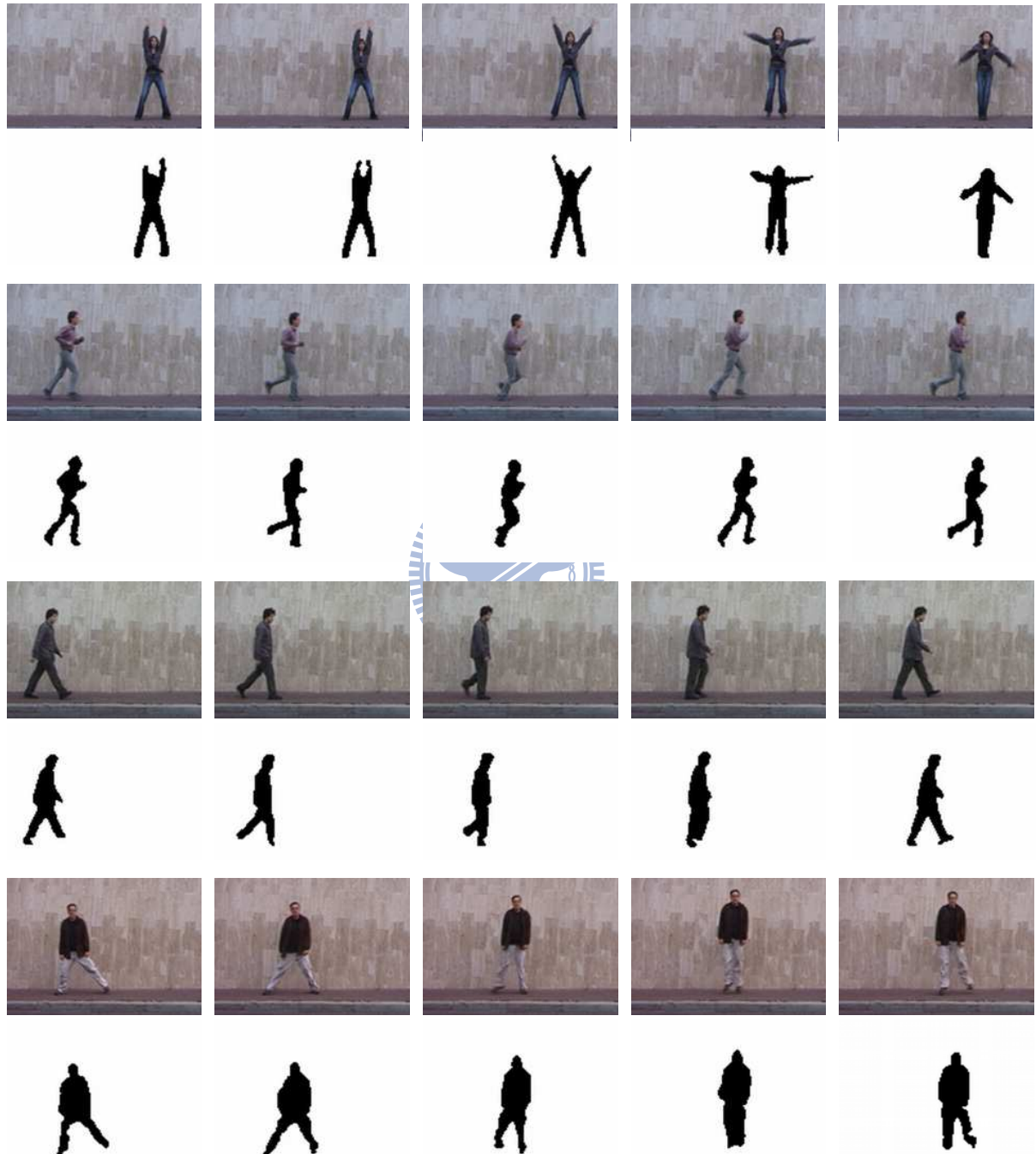
Fig. 4.4 Examples of video sequences and extracted silhouettes from Weizmann's database [14].
