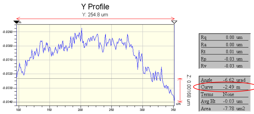
Figure 4-1. Surface profile of the mirror plate of sample A, (a) 3-D profile, (b) cross section schematic of the mirror plate, (c) 2-D profile, (d) 2D profile of the flat area along A-B and (e) 2D profile of the flat area along C-D (continued).
