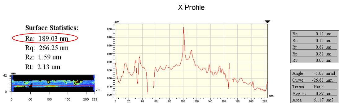
Figure 4-9. Surface profile of the torsional spring of sample C.
