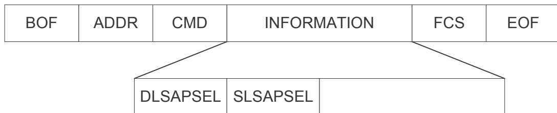
Figure 44. IrDA LMP Frame Structure.
