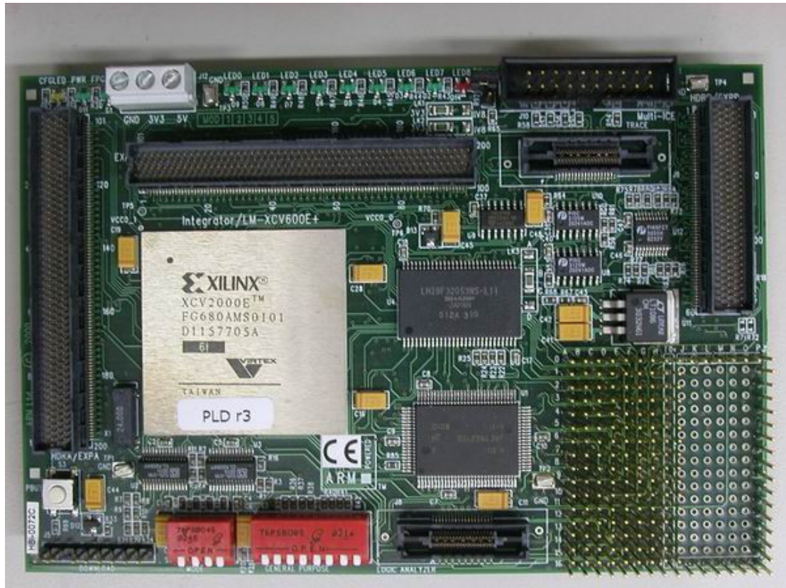
Figure 4. ARM Logic Module with Xilinx XCV2000E FPGA
