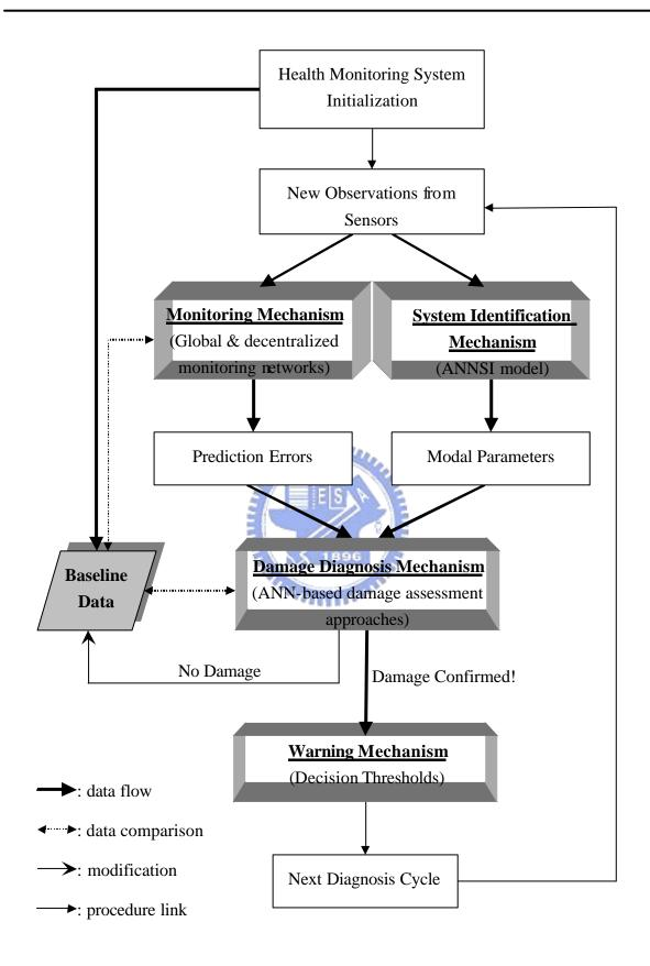
Figure 8.1 Operation of the integrated health monitoring system
