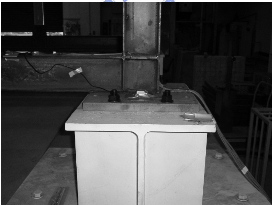
Figure 6.8 Accelerometer at the base of the test frame
