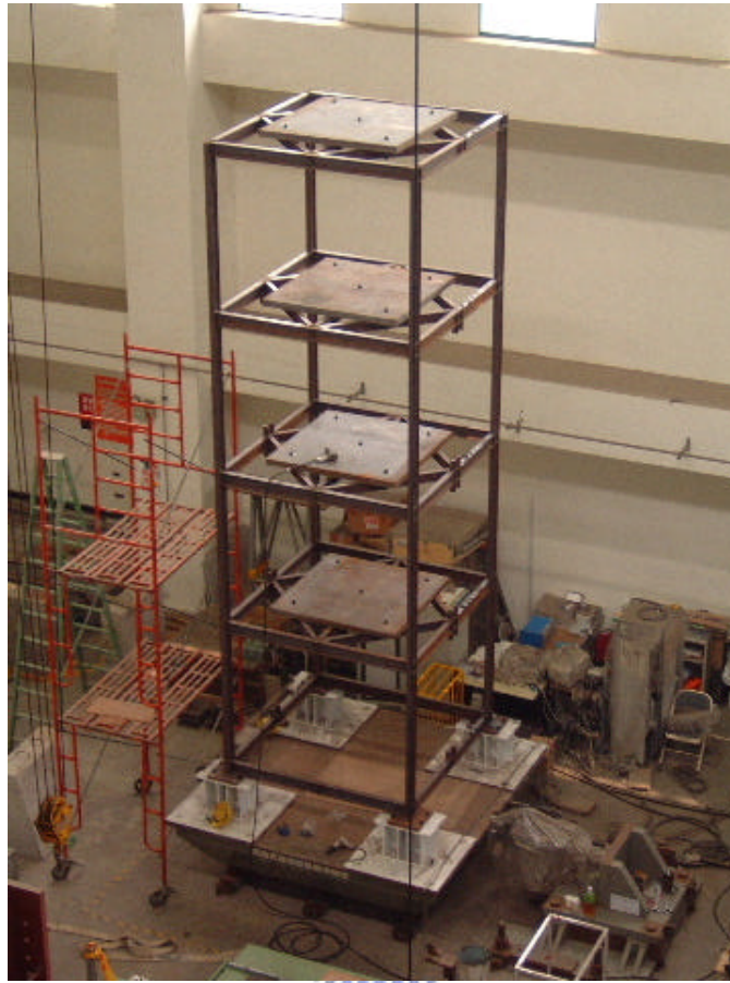
Figure 6.5 A photo of the four-story clear frame
