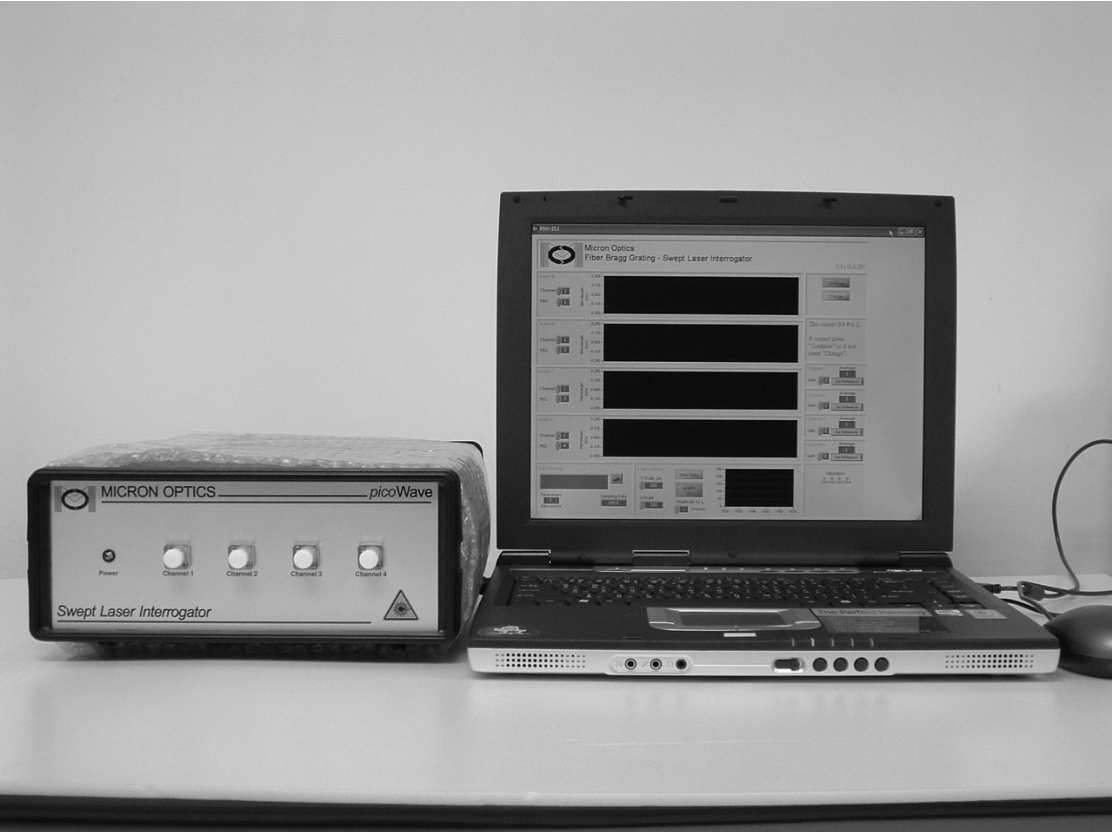
Figure 6.11 FBG data acquisition system
