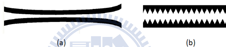
Figure 2.3-1 Examples of non-uniform couplers (a) Smooth-edge coupler (b) wiggly coupler
