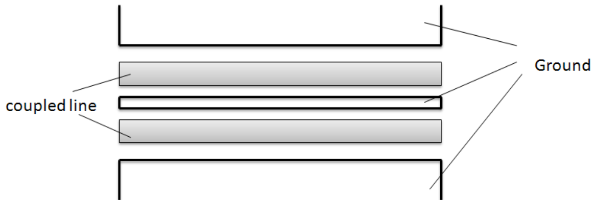
Figure2.4-2 Second method to achieve loose-coupling CPW coupler
