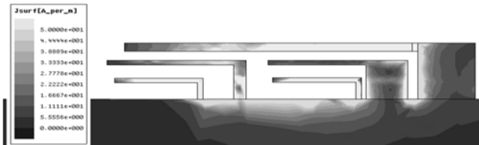
Figure 4.12: Current distributions of the proposed penta-band monopole antenna at 0.84 GHz.
