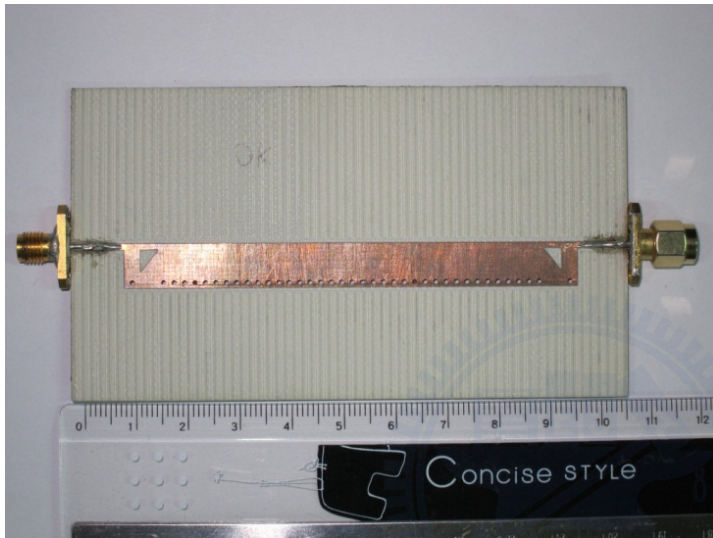
Fig 4.11 The fabricated HMSIW LWA prototype
