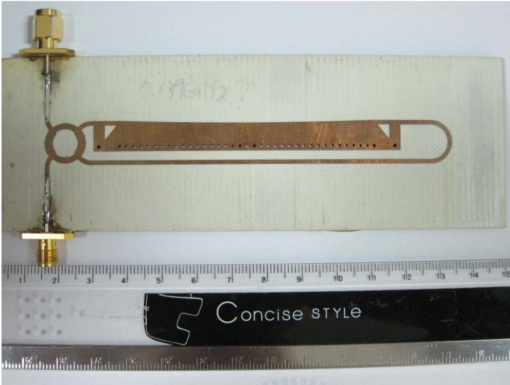
Fig 6.10 The fabricated LWA integrated with the feed-back network
