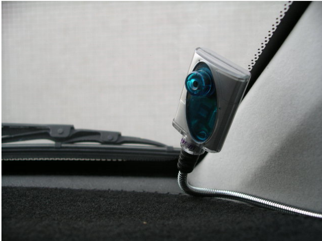
Fig. 5-18 The USB CCD mounted behind the right front windshield
