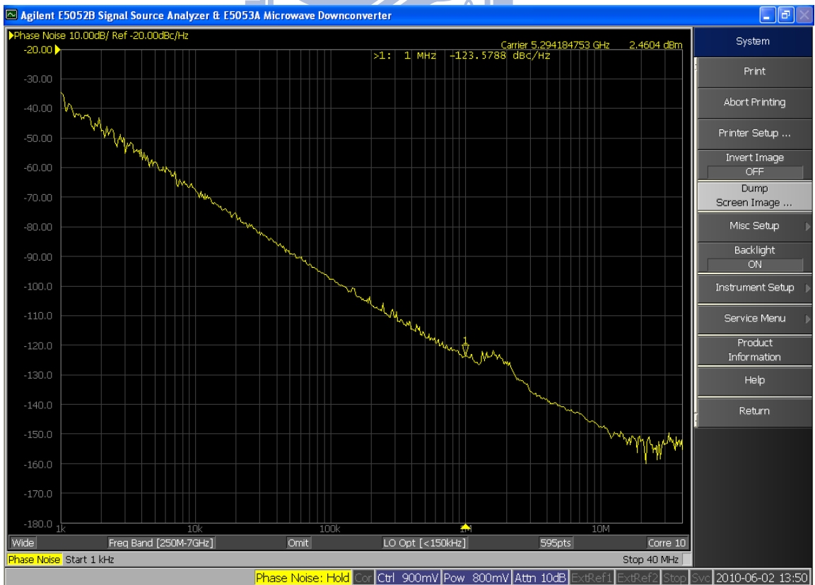
Fig. 3 - 26 Measured phase noise of the proposed self-switching biased QVCO at f_0= 5.29\text{GHz}
