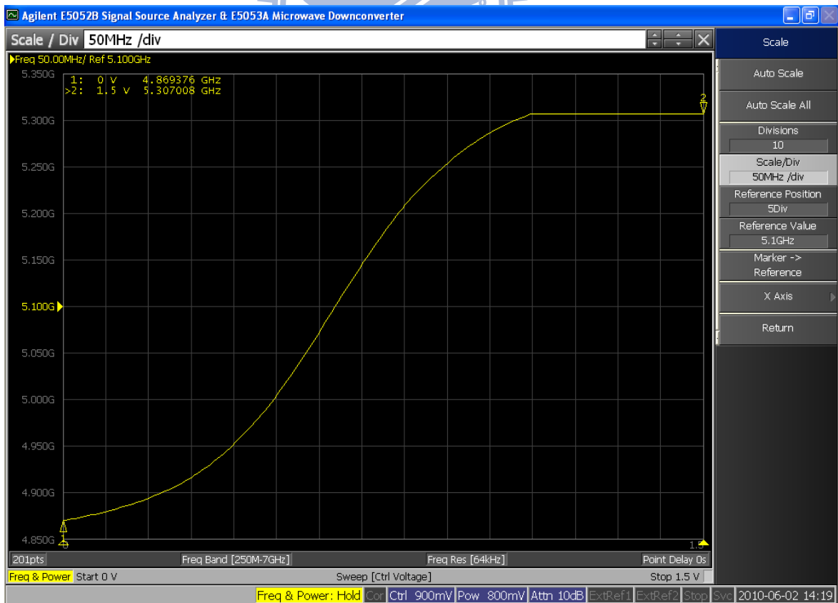
Fig. 3 - 28 Measured tuning range of the proposed self-switching biased QVCO
