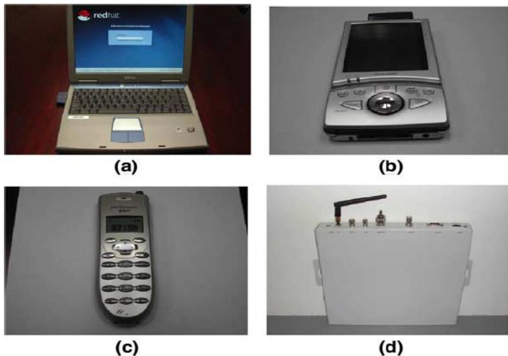
Figure 1.3 Examples of mesh clients: (a) Laptop, (b) PDA, (c) Wi-Fi IP Phone (d) Wi-Fi RFID Reader.
