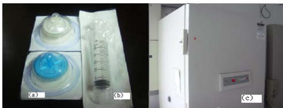
圖3.8 (a)針頭式過濾器、(b)針筒、(c)負80°C冰箱
