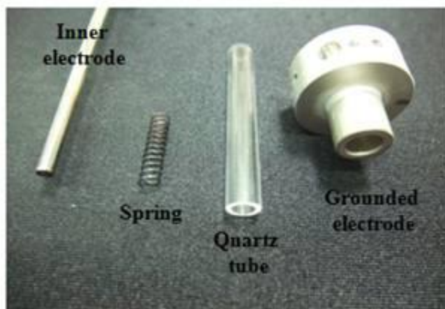
Figure 2.4 The schematic diagram of electrode configuration.
