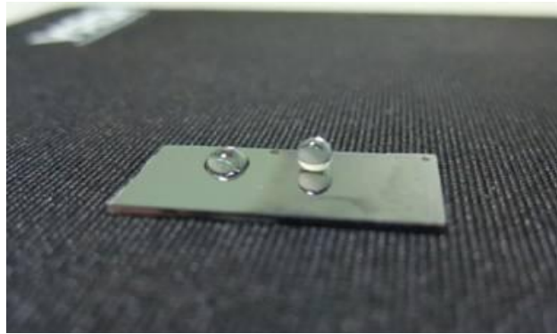
Figure 3.28 Image of super-hydrophobic surface.
