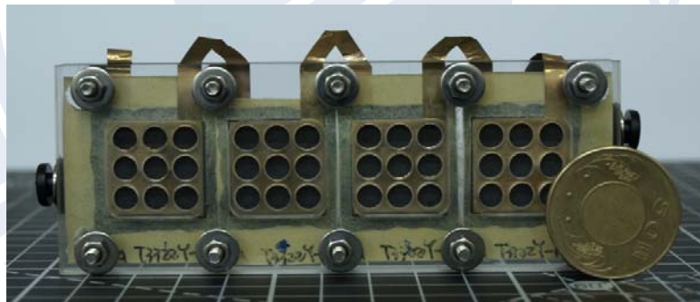
Fig. 3.22 Cathode Side of the PEMFC Stack
