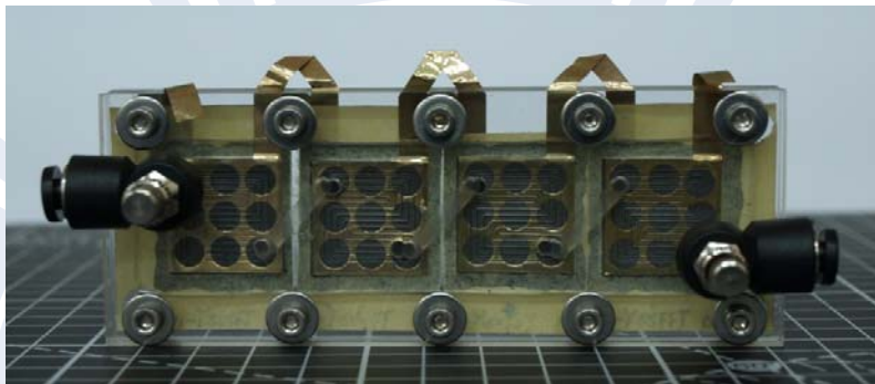
Fig. 3.21 Anode Side of the PEMFC Stack
