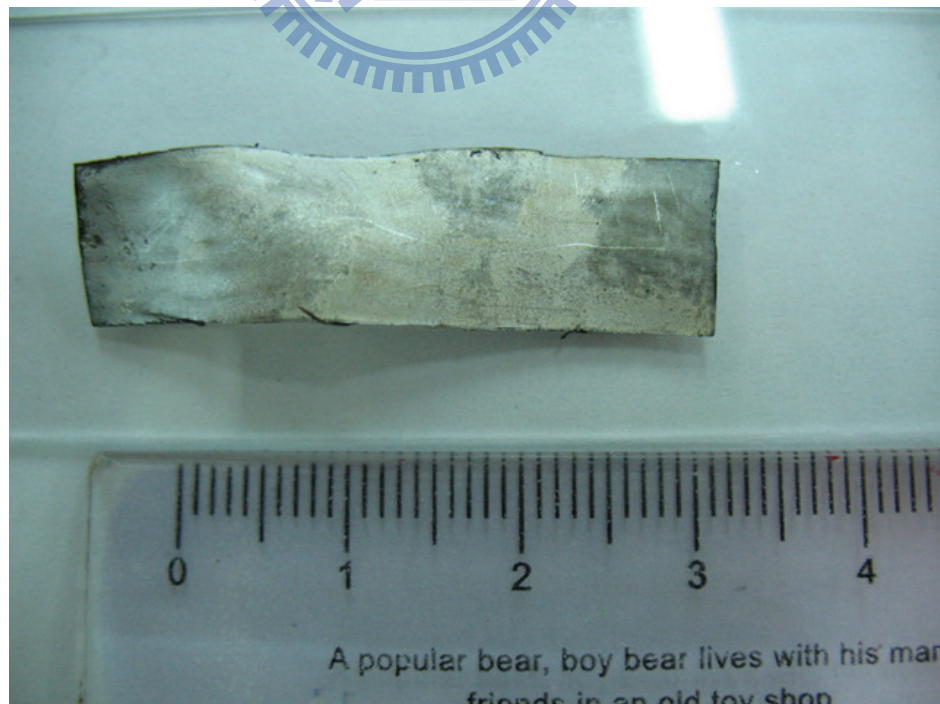
Figure 5.10 The 1 mm thick self-made membrane was coated with silver.
