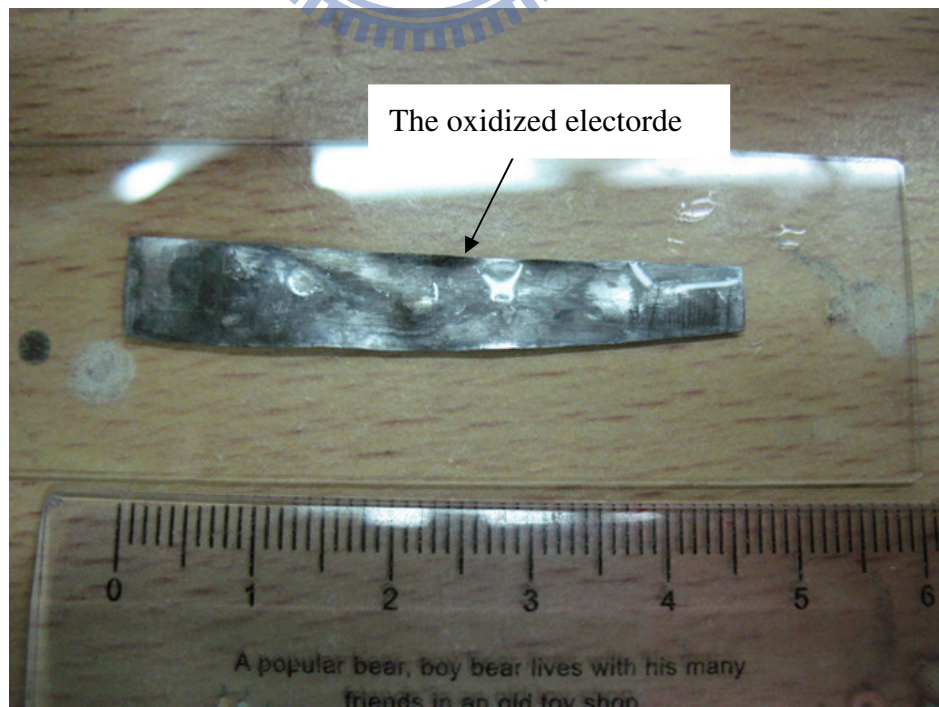
Figure 6.5 the sample performed the largest displacement After the actuation, the sample was broken due to the electrolysis of H_2O , as shown in figure 6.6. And the copper electrode on the sample clip was also electrolyzed, as shown in figure 6.7.
