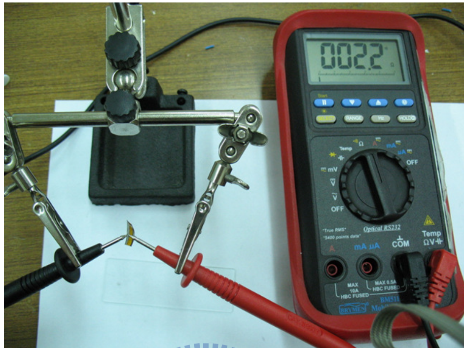
Figure 5.5 the measurement of the marginal electrode resistance of the second kind electrode distribution of first type membrane
