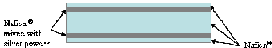
Figure 4.51 the sandwich structure of vertical casting IPMC
