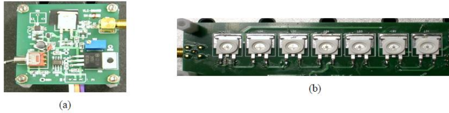
圖 3-4 (a)單顆 LED 燈構造(b)LED 燈陣列[14]
