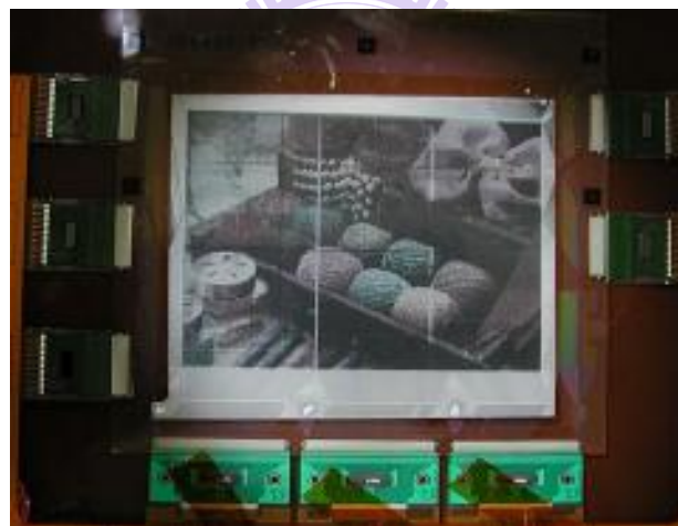
Fig.4-1. The e-paper using oxide semiconductor TFT fabricated on flexible substrate.
