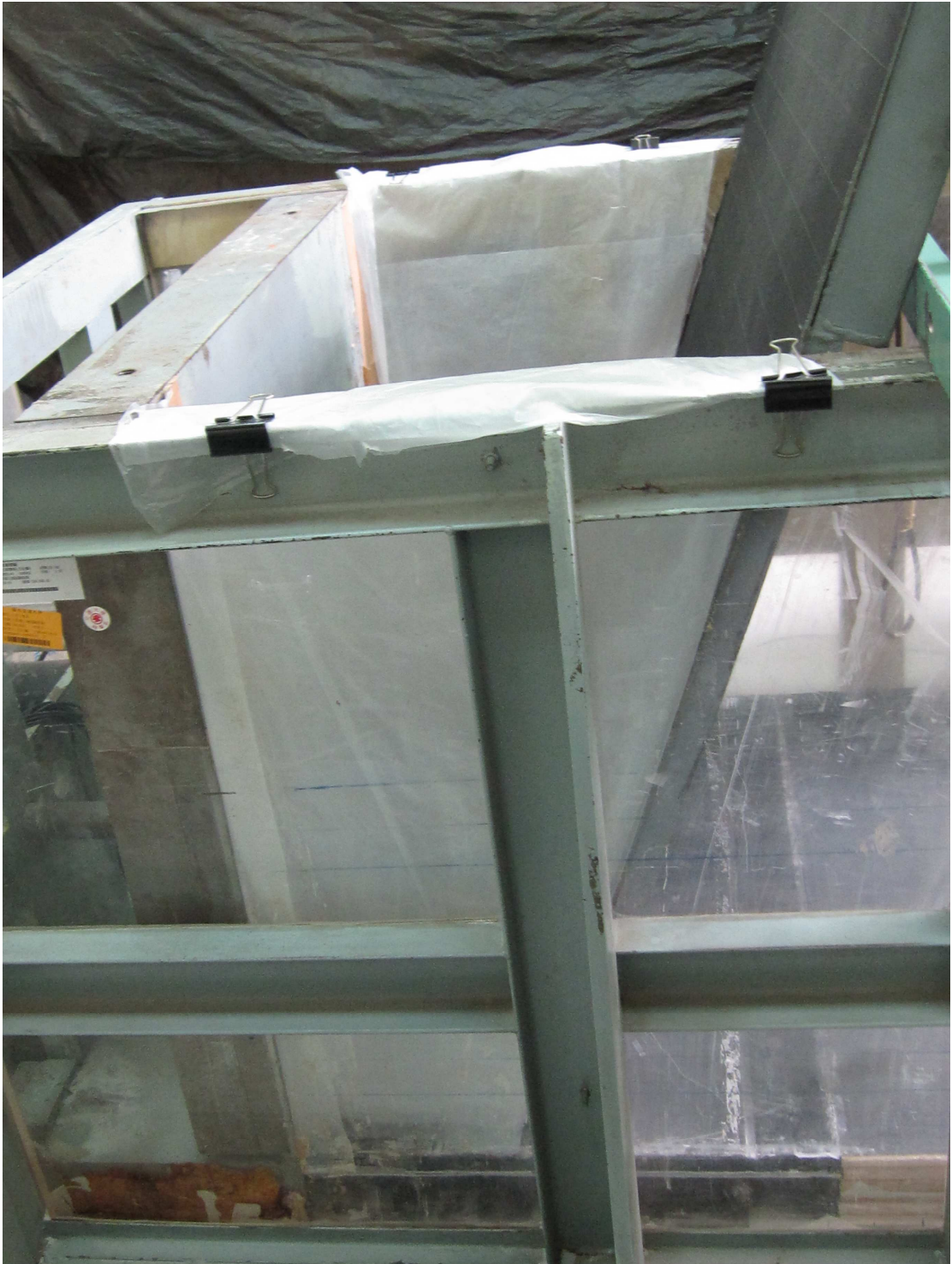
Fig. 6.32. Model wall test with interface spacing b = 250 mm and \beta = 70^\circ
