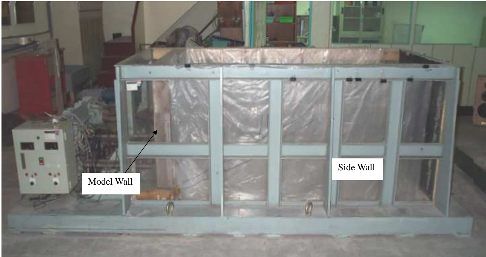
Fig. 3.7. Plastic-sheet on each sidewall
