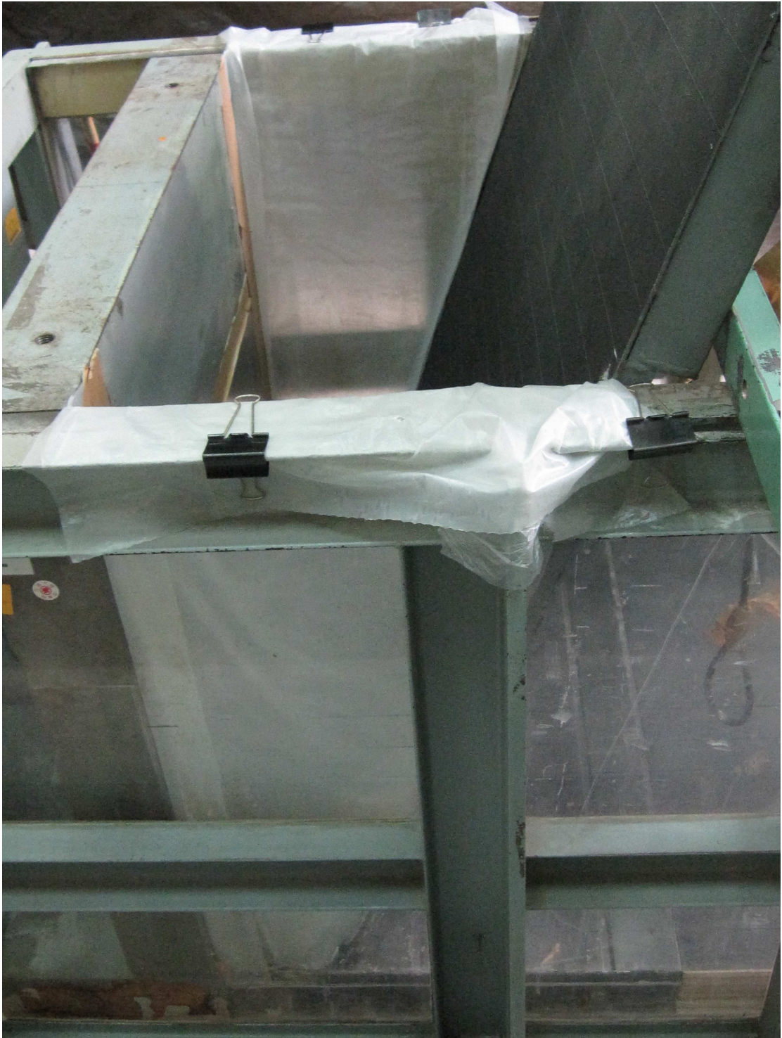
Fig. 6.12. Model wall test with interface spacing b = 150 mm and \beta = 70^\circ
