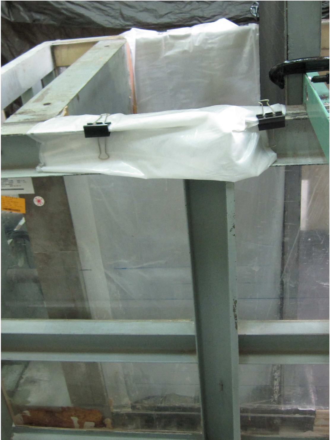
Fig. 6.51. Model wall test with interface spacing b = 500 mm and \beta = 90^\circ
