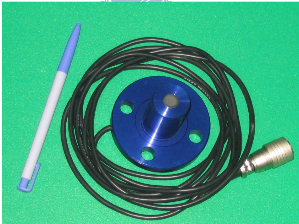
Fig. 3.6. Soil pressure transducer (Kyowa PGM-0.2KG)
