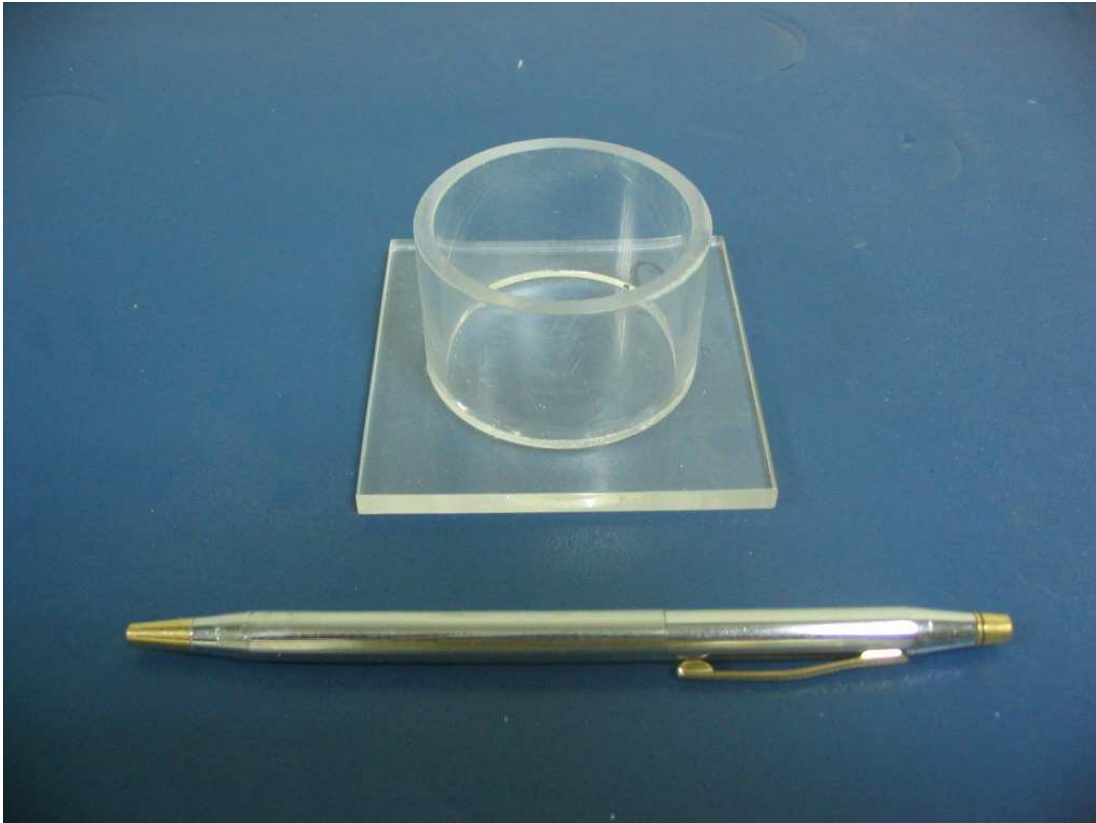
Fig. 5.17. Soil-density cup (after Chien, 2007)
