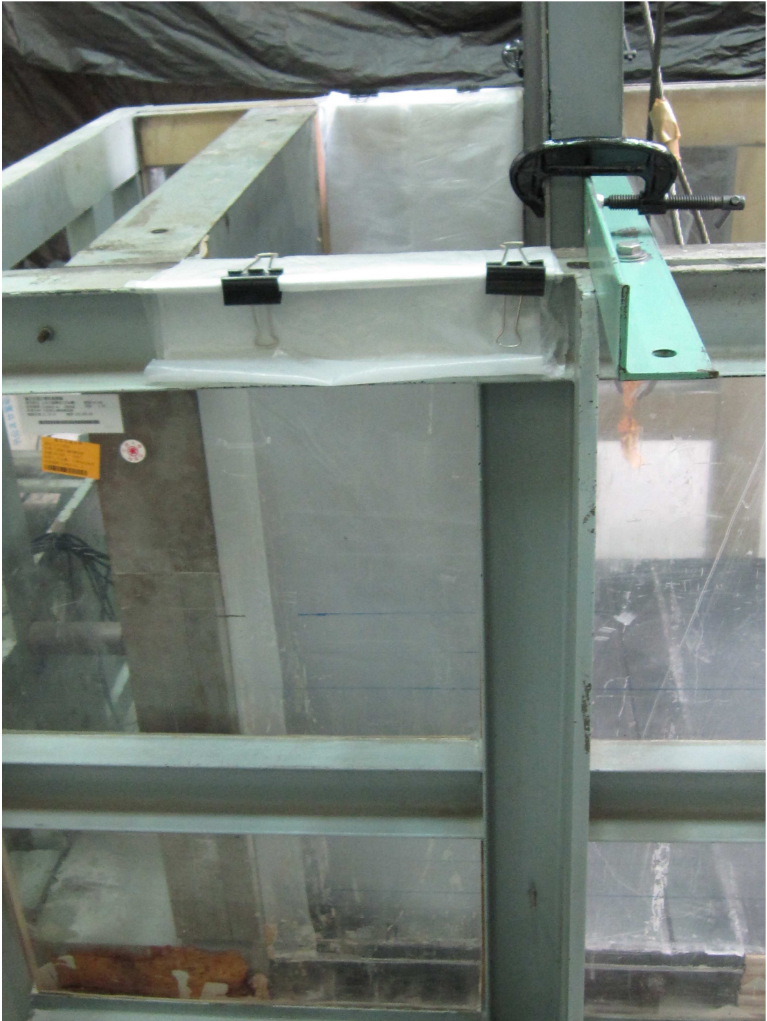
Fig. 6.41. Model wall test with interface spacing b = 350 mm and \beta = 90^\circ
