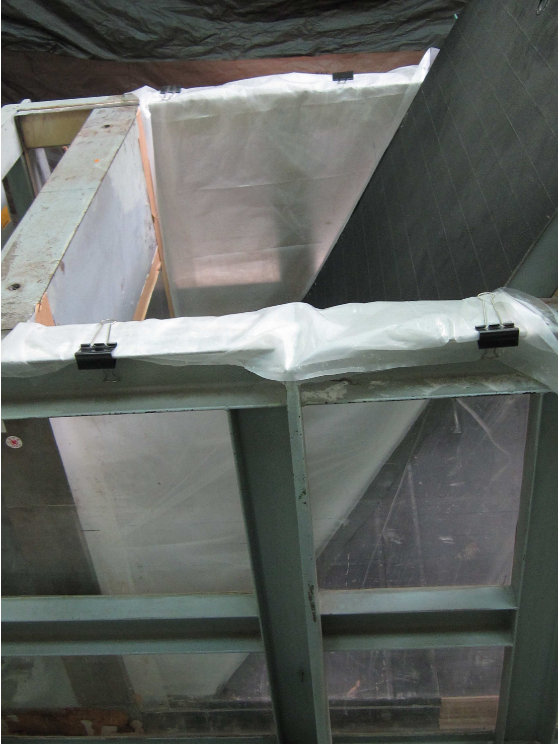
Fig. 6.15. Model wall test with interface spacing b = 150 mm and \beta = 60^\circ
