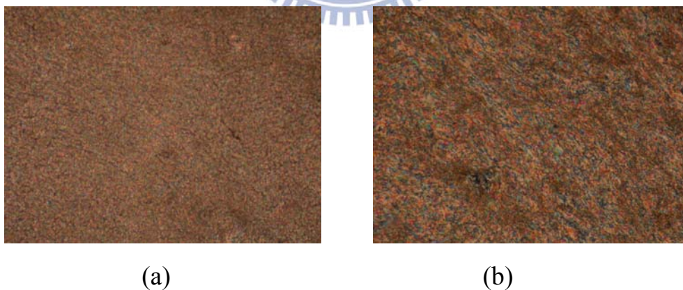
Fig. 3-1-2.1 POM textures at the cooling process: (a) the polar smectic phase of complex SiA-PyBVF 14 at 127 °C; (b) at 100 °C
