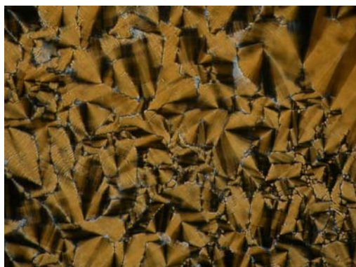
Fig. 3-1-2.2 POM textures of SiA-PyBVF 14 by applying electric fields ( V_{pp} = 300 \text{ V} )
