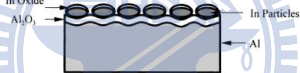
Fig. 2-11 Schematic representation of the ordered array of In nano-particles.
