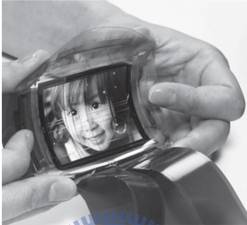
Figure 2. 2. Photograph of the OTFT-driven OLED display under operation
