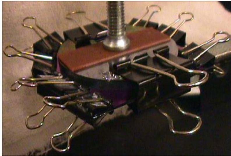
Figure 3. 4. C-clamp and small clamps for fixing four point bending sample
