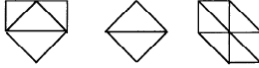
Figure 1.4.2: Domain \omega_T, \omega_E and \omega_x
