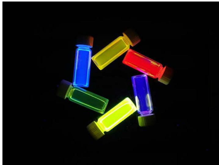
Figure 1.8: Emission color under UV illumination for colloidal CdSe/ZnS QDs with various sizes [14].
