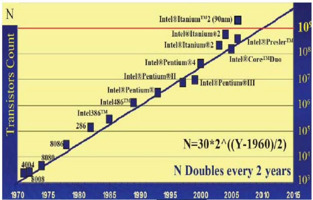
Fig. 1-1 The transistors count of CPU increases with year, and doubles every 2 years [1].
