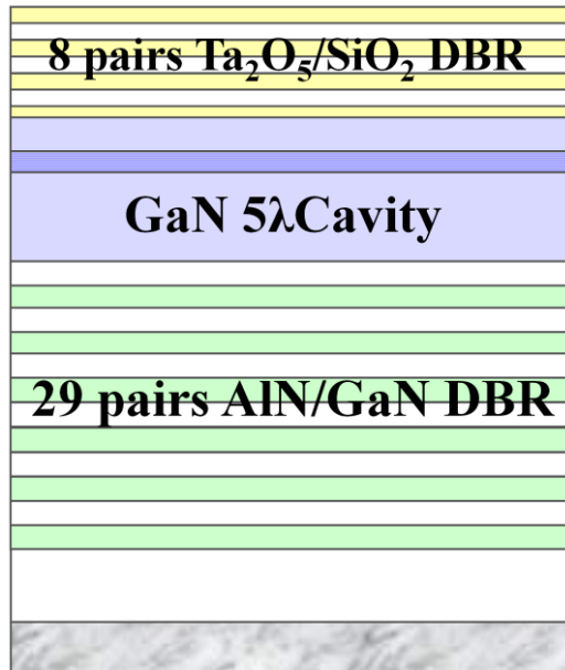
Fig. 4.1 The schematic diagram of the optical pumped VCSEL structure
